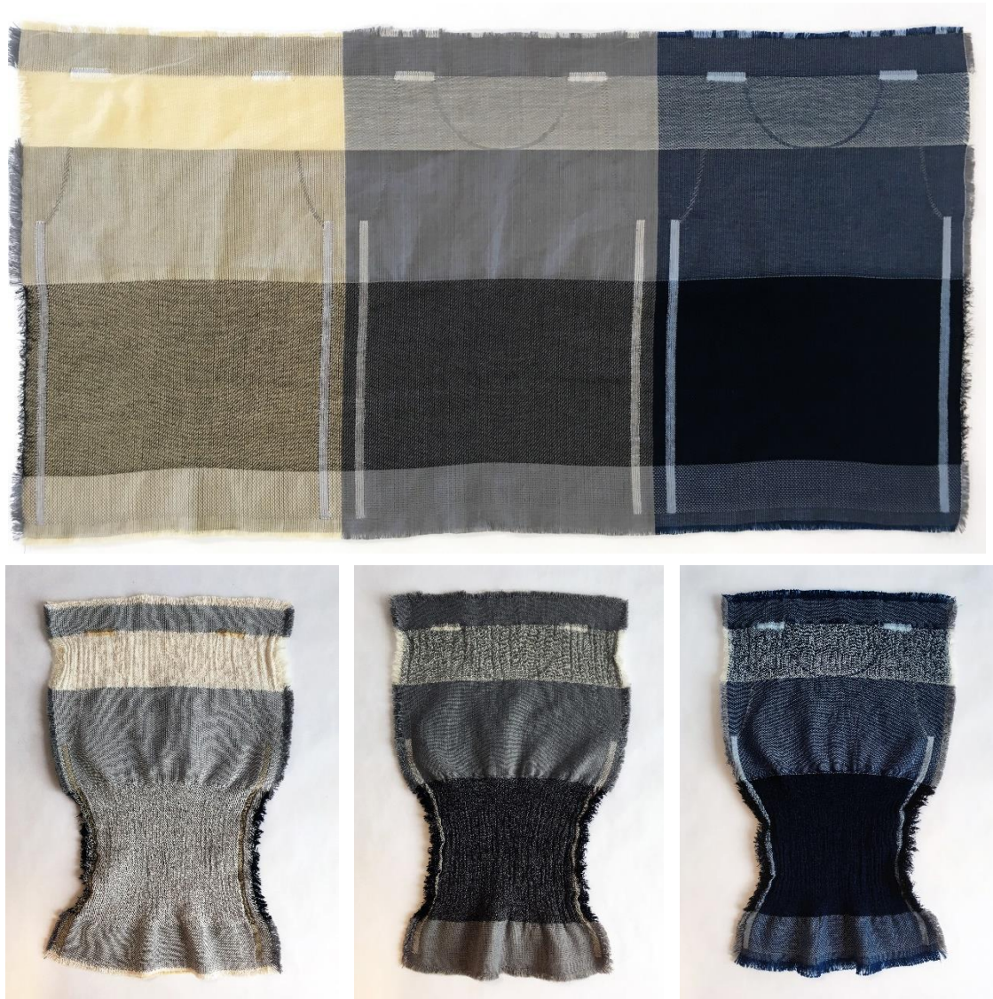
Figure 6.16. A Jacquard sleeveless top when cut off the loom (top) and after the finishing process (bottom)
