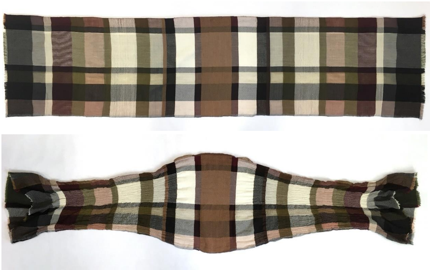
Figure 6.13. A tubular jumper/jacket when cut off the loom (top) and after the finishing process (bottom)
