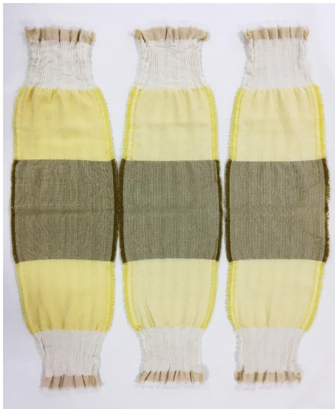
Figure 6.19. A Jacquard tubular jumper/jacket when cut off the loom (top) and after the finishing process (bottom)
