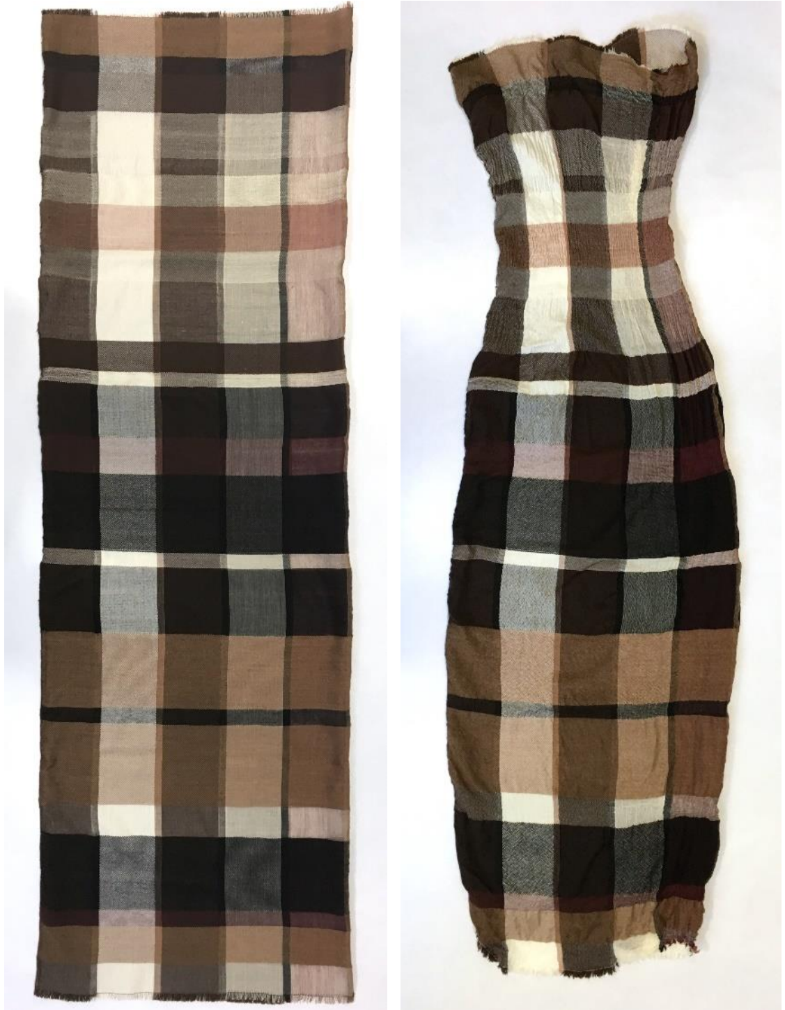
Figure 6.7. A tube dress when cut off the loom (left) and after the finishing process (right)
