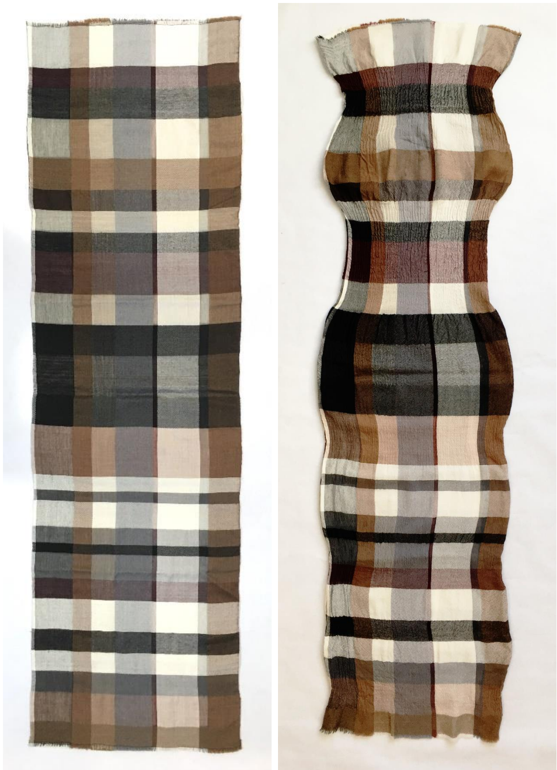
Figure 6.10. A long sleeveless dress when cut off the loom (left) and after the finishing process (right)
