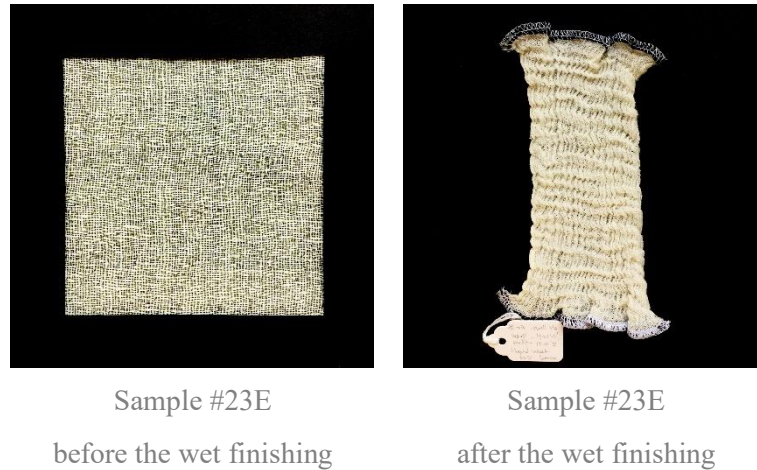
Figure 5.12. Comparison of sample #23E before and after the wet finishing process
