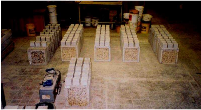
Fig. 1 Concrete substrate surfaces obtained using either RRH or an electric hammer.
