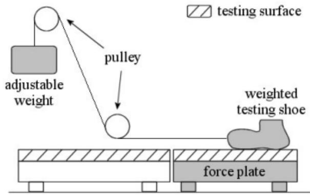
Figure 1 – Pulley system in mechanical slip resistance test
