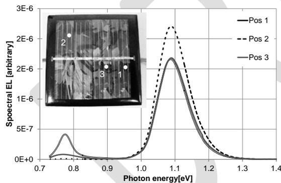
Figure 4: Localised spectral EL measurements of mc-Si sample at different points as indicated
