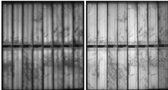
Figure 3: EL images of mc-Si single cell; left: excitation current at  $1xI_{sc}$ ; right: current at  $0.2xI_{sc}$ ; images are normalised, in absolute terms the right image is much darker due to the lower injection current
