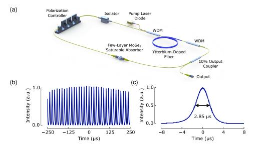
Fig. 4. Yb:fiber Q-switched laser: (a) cavity schematic; (b) output pulse train at 65.0 kHz repetition rate; (c) pulse profile with 2.85 µs duration for 8.0 mW average output power.
