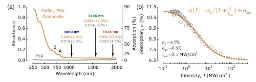
Fig. 3. Few-layer MoSe<sub>2</sub>-PVA SA characterization: (a) linear optical absorption, with highlighted absorption values at the operating wavelengths of our MoSe<sub>2</sub>-based Q-switched lasers; (b) nonlinear optical absorption (at 1566 nm) measured by a Z-scan technique and well fitted by a two-level SA model [46],where  $\alpha$  is absorption, I is incident intensity,  $\alpha_s$  is modulation depth,  $\alpha_{ns}$  is nonsaturable absorption and  $I_{sat}$  is saturation intensity.
