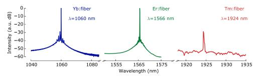
Fig. 7. Spectra for Q-switched operation of few-layer  $MoSe_2$  Q-switched Yb- and Er- and Tm-doped fiber lasers; the Yb and Er spectrum were measured using an optical spectrum analyzer (0.02 nm resolution), while the Tm spectrum was measured on a spectrometer ( $\sim$ 0.1 nm resolution).
