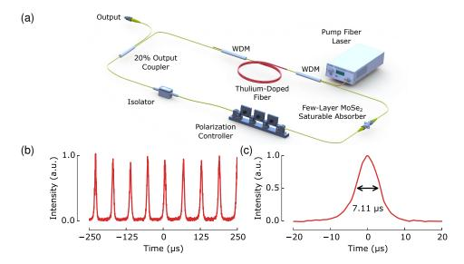
Fig. 6. Tm:fiber Q-switched laser: (a) cavity schematic; (b) output pulse train at 16.9 kHz repetition rate; (c) pulse profile with 7.11 µs duration for 0.79 mW average output power.
