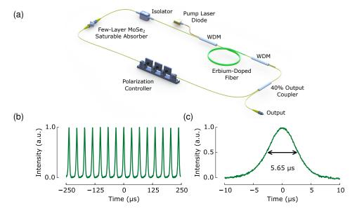
Fig. 5. Er:fiber Q-switched laser: (a) cavity schematic; (b) output pulse train at 29.4 kHz repetition rate; (c) pulse profile with 5.65  $\mu s$  duration for 24.5 mW average output power.
