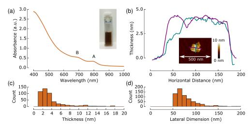
Fig. 1. (a) Linear optical absorption of MoSe<sub>2</sub> flakes in a 10% (v/v) dispersion, showing characteristic excitonic peaks (A & B) (inset: photograph of the diluted dispersion). AFM characterization of MoSe<sub>2</sub> flakes: (b) AFM image of a typical flake and two thickness profiles; (c) distribution of flake thicknesses; (d) distribution of lateral flake dimensions.
