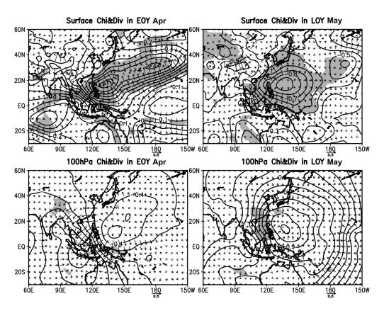
Figure 9. Composite anomalies of velocity potential (contour, unit: m s<sup>-1</sup>, scaled by 10<sup>6</sup>) and divergent wind (vector, unit: m s<sup>-1</sup>) at surface and 100h hPa levels in (left) April of EOY and (right) May of LOY. Shading indicates significance at the 95% confidence level for velocity potential or divergent wind. 166x131mm (300 x 300 DPI)
