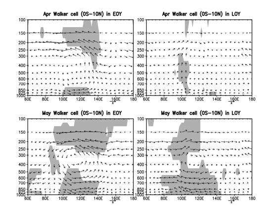
Figure 8. Composite anomalies of the zonal-vertical circulation of the equatorial region (0-10N) prior to the SCSSM onset in EOY (left panel) and LOY (right panel). The vertical component of the vectors is the pressure vertical velocity (unit: Pa s<sup>-1</sup>, scaled by -100), and the horizontal component is the zonal component of the wind. Shading indicates significance at the 95% confidence level for vertical velocity. 177x142mm (300 x 300 DPI)
