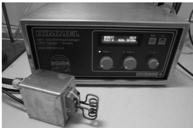
Figure 11. An inductive system used for the machine-assisted heating of a continuous flow reactor column. Reprinted from [54a].
