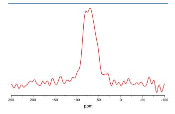
**Figure 13.** <sup>19</sup>F $\rightarrow$ <sup>13</sup>C CP-MAS NMR spectrum of HBM CCN-CuF<sub>2</sub>. No signal was present in the spectrum when the <sup>19</sup>F CP pulses were removed.
