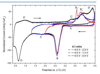
**Figure 3.** First sweeps in the cyclic voltammograms of a CCN-CuF<sub>2</sub> electrode for different potential windows (red, 4.5-2.0 V; blue, 4.5-1.3 V; black, 4.5-0.4 V) with a scan rate of 0.1 mV/s. The current is normalized per gram of active material.
