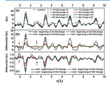
**Figure 11.** (a) Select in situ PDFs for CCN-CuF<sub>2</sub> measured for four cycles. Only the PDFs for the beginning and the end state of each cycling steps are shown. Differential PDFs on each discharge (b) and charge (c) step, obtained by subtracting the PDF of the end state from the PDF of the beginning state of each cycling step. Black and red arrows indicate the atom pairs corresponding to the Cu and CuF<sub>2</sub> phases, respectively.
