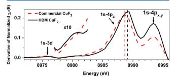
**Figure 6.** First derivatives of the normalized Cu K-edge XANES spectra of commercial  $\text{CuF}_2$  (red dash) and HBM CCN- $\text{CuF}_2$  (black solid). The inset shows a magnification (×10) of the spectra in the same energy region. An additional absorption peak is present at around 8980 eV in HBM CCN- $\text{CuF}_2$  suggestive of the presence of Cu<sup>+</sup> components.
