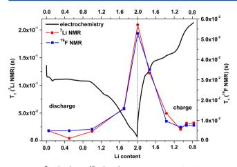
**Figure 15.** <sup>7</sup>Li (red) and <sup>19</sup>F (blue)  $T_1$  measurements for the samples shown in Figure 14. The electrochemical potential profile is shown for comparison.
