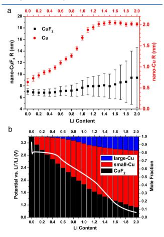
**Figure 9.** (a) The evolution of the particle sizes from the initial structure refinement (no particle size constraints applied) and (b) the phase mole fractions from the final structure refinement against the PDFs on the first discharge shown in Figure 8. The white potential profile in part b illustrates the corresponding potential curve for the in situ battery.
