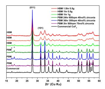
**Figure 1.** Laboratory XRD patterns for commercial CuF<sub>2</sub> and CCN-CuF<sub>2</sub> nanocomposites prepared under various conditions. The two main CuF<sub>2</sub> reflections, (011) and (101), are labeled. The two reflections marked with asterisks at low angles correspond to impurity phases. The reflection at 18.8°  $2\theta$  is assigned to Cu(OH)F and/or CuF<sub>2</sub>·2H<sub>2</sub>O. HBM, high-energy ball mill; PBM, planetary ball mill.
