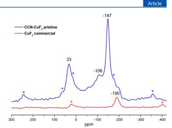
Figure 12. Normalized  $^{19}\mathrm{F}$  MAS NMR spectra of the commercial CuF\_ (red) and HBM CCN-CuF\_ (blue). Signals marked with asterisks are spinning side bands. No  $^{19}\mathrm{F}$  signal background from the rotor is observed.
