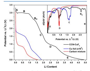
**Figure 4.** Potential profiles for batteries using CCN-CuF<sub>2</sub> (black), Cu foil (blue), and carbon mixture (red) as cathode materials discharged to 0 V. The capacity from Cu foil has been scaled by  $10^3$  for a better comparison. The inset shows a dQ/dV plot converted from the potential profiles.
