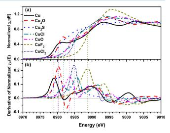
**Figure 5.** (a) Normalized Cu K-edge XANES spectra of Cu metal and Cu reference compounds (Cu<sub>2</sub>O, Cu<sub>2</sub>S, CuCl, CuO, CuF<sub>2</sub>, CuCl<sub>2</sub>). (b) First derivatives of the normalized Cu K-edge XANES spectra shown in part a. The positions of the edge energies of each reference material are marked with dotted lines.
