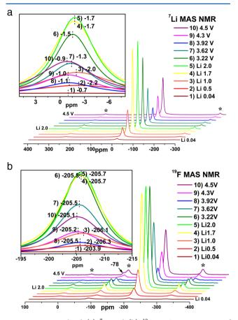
**Figure 14.** Normalized (a) <sup>7</sup>Li and (b) <sup>19</sup>F MAS NMR spectra of cycled CCN-CuF<sub>2</sub>. Signals marked with asterisks are spinning side bands. The insets show the overlay plots of the isotropic resonances of the corresponding spectra. Numbers in the insets are the values of the chemical shifts. ("Li *x.x*" represents the specific capacity on discharge; "*x.x* V" refers to the potential on charge where the samples were collected for measurement.)
