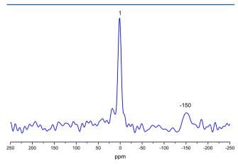
Figure 16.  $^{31}$ P MAS NMR spectrum of fully discharged CCN-CuF<sub>2</sub> (Li = 2.0).
