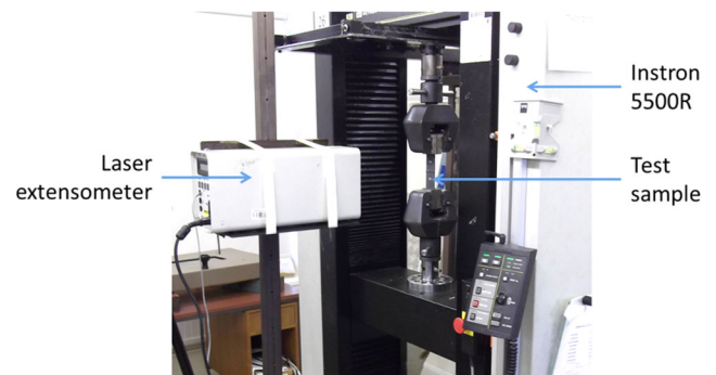
Fig. 4 Tensile test setup used for CMT Cu welded samples
