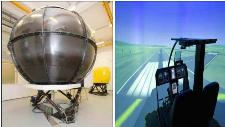
Fig. 2 External and interior views of the HELIFLIGHT-R flight simulator
