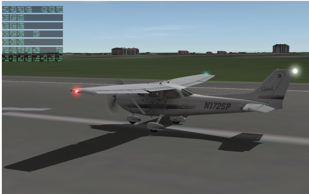
Figure 5.2: Cessna 172SP in X-Plane with failure on the LEFT WING 1 part. The left aileron is stuck at a deflection.
