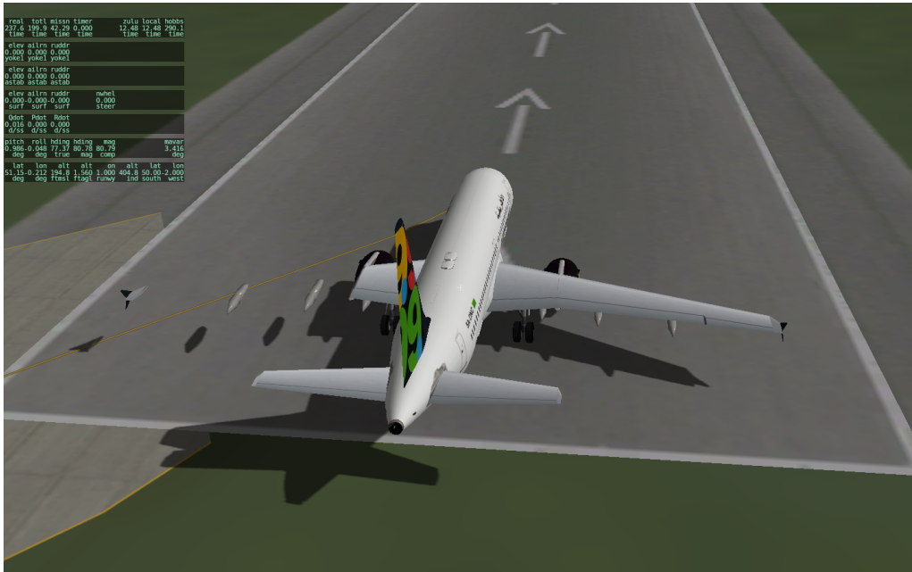
Figure 5.3: Airbus A320 in X-Plane with failure on the LEFT WING 2 part. The WING 2 section of the aircraft appears to be removed or destroyed.
