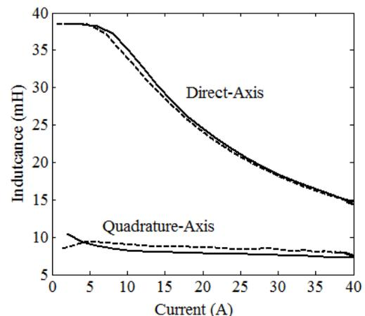
Fig. 10. Experimental (dashed) and finite element (solid)  $dq$ -axis inductance curves. The curves in the  $d$ -axis show a very close match and the  $q$ -axis inductance shows a lower degree of agreement due to parasitic end effects not considered by the lumped leakage inductance. Experimental results however show that the finite element model will accurately predict machine performance. Figure 11 shows the prototype rotor used during measurements and Figure 12 shows the experimental setup.
