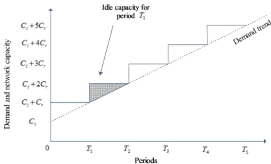
**Figure 1: Demand growth and network capacity enhancement**
