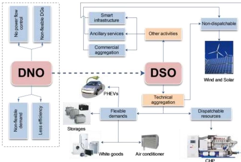
**Figure 2: A future distribution system operator (DSO) model**
