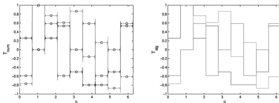
FIGURE 6.  $\mathbf{T}_{num}$  versus  $\mathbf{T}_{alg}$ , for  $M = 3$ , at  $T_{1,3} = \frac{2\pi}{27}$ .  $T_1$  appears in blue,  $T_2$  in green,  $T_3$  in red. In  $\mathbf{T}_{num}$ , the Gibbs phenomenon is clearly visible. The black circles denote the points chosen for the comparisons.
