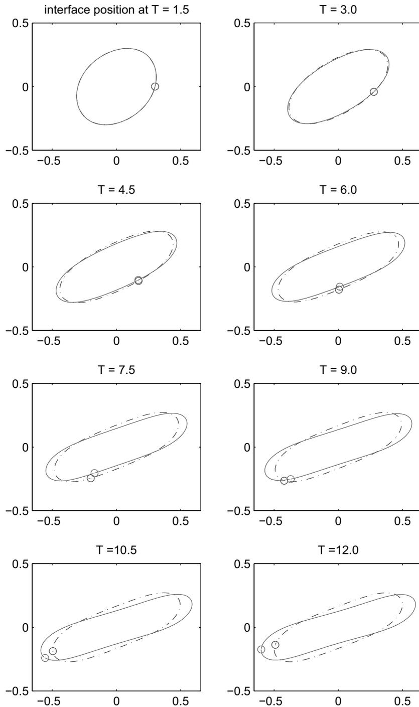
Figure 2: The interface positions of clean (denoted by "-.") and soluble (denoted by "-.") interfacial flows for a drop under shear flow.
