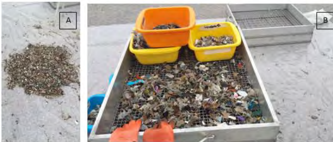
Fig. 7: Merceologic analysis. On the left side (A) there is the picture of the undersieve ( < 20\text{mm} ). On the right side is shown how was done the merceologic analysis
