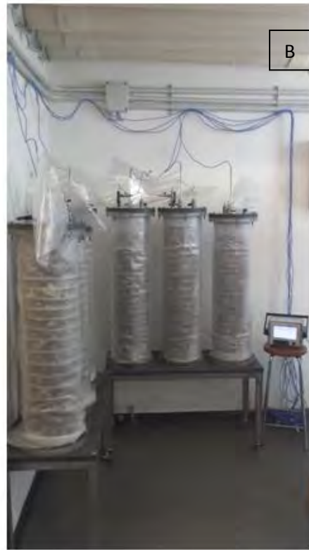
Fig. 3: Steps required for the creation of the insulating system. In the picture A can be seen the PVC pipe wrapped around all the columns. Picture B shows the two layers of pluriball and the picture on the right side the complete “jacket” with the aluminum foil
