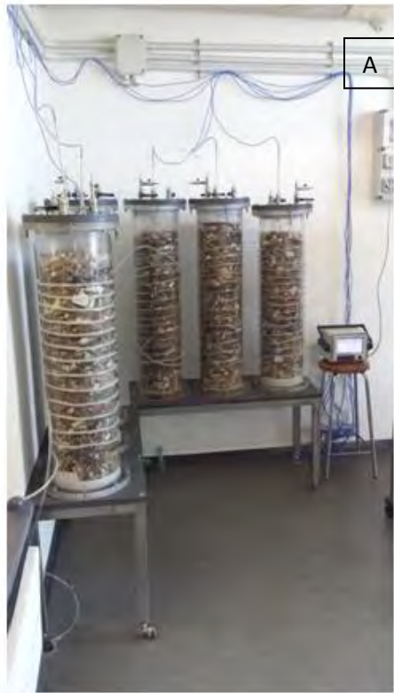
Fig. 3: Steps required for the creation of the insulating system. In the picture A can be seen the PVC pipe wrapped around all the columns. Picture B shows the two layers of pluriball and the picture on the right side the complete “jacket” with the aluminum foil
