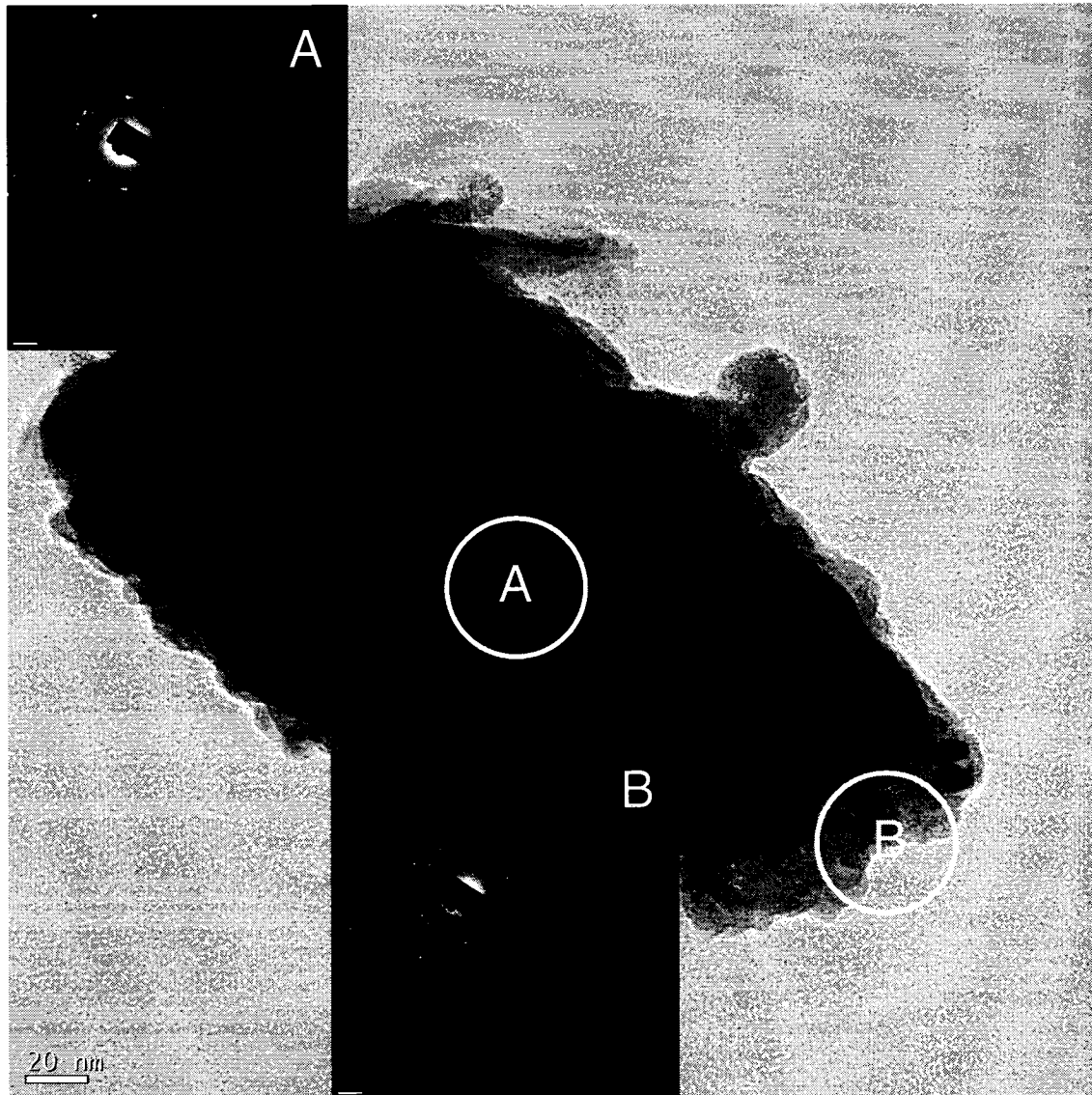
Figure 4.52: TEM image of a second particle to further study the absence of amorphous structure in the as-milled 40Al-25Mg-35Zr alloy.
