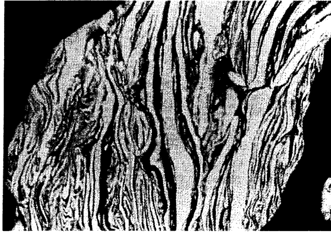
Figure 2.3: Resulting layered structure from milling [10].
