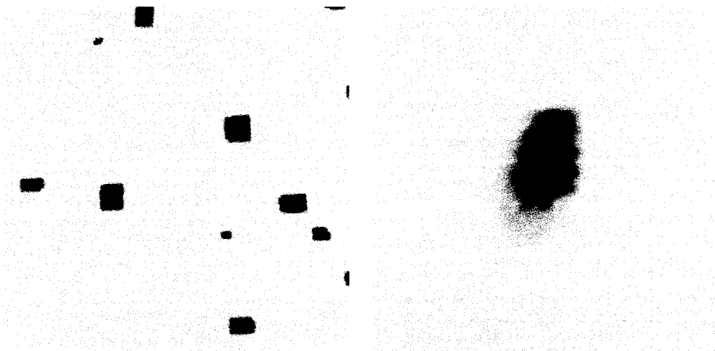
Figure 3.7: The smallest observed pits for samples prepared at 250 \text{ }^\circ\text{C} are 3.0 \pm 0.6 \text{ nm}^2 in size: (a) 100 \text{ nm} \times 100 \text{ nm} ( \Delta f = -3.6 \text{ Hz} ), (b) 10 \text{ nm} \times 10 \text{ nm} ( \Delta f = -10.2 \text{ Hz} ).
