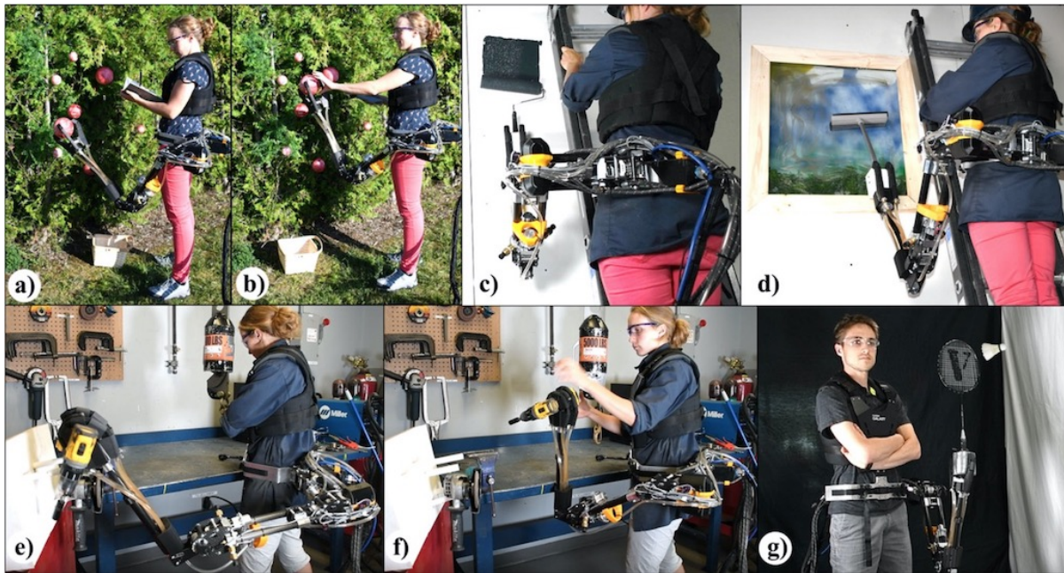
Figure 2.23: Waist-Mounted Extra Arm. This shows a number of example tasks used to test the robot: fruit picking (a,b), painting (c) window cleaning (d), assistive power tool handling (e,f), hands-free badminton [226]
