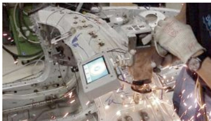
Figure 2.18: Intelligent Welding Gun in operation. Reflective markers enable localisation and a mounted display delivers feedback to the welder Echtler et al. [47].
