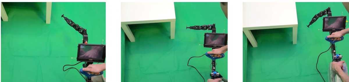
Figure 2.3: 6-DoF handheld robot pointing its tip towards the point it needs to be positioned in order to indicate goal direction. In this example, an LCD display is used for visual feedback [59].
