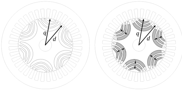
Fig. 8. Structures of a SynRM and a PMa-SynRM.
