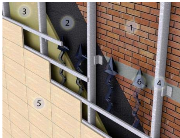
Figure 1. Image of layers of a ventilated façade system: 1. Inner wall; 2. Breathable and waterproof sheet; 3. Continuous insulating layer; 4. Load-bearing structure; 5. Joined building wall; 6. Ventilated air gap.
