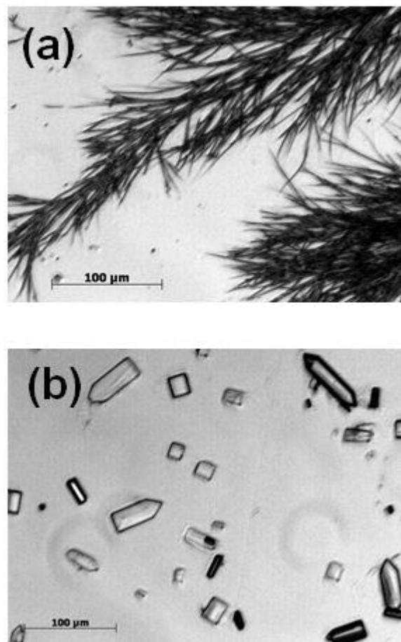
**Figure S3.** Optical micrographs of (a) tubes organized in dendritic branches and (b) FF monocrystals obtained at 4 °C for FF dissolved at a final concentration of 1 mg/mL in DMF:water 1:4 and DMSO:water 1:4, respectively.
