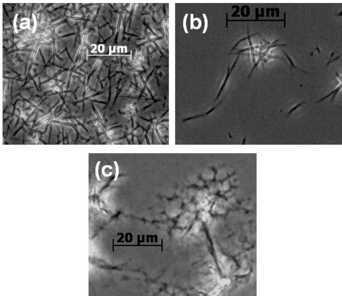
**Figure S1.** Optical micrographs of tubes obtained at 4 °C for FFFF dissolved at a final concentration of 0.5, 0.1 and 0.05 mg/mL in DMF:water 1:9, 1:49 and 1:99, respectively.
