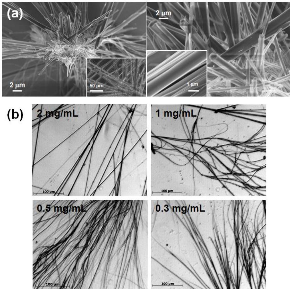
**Figure S2.** (a) Low and high magnification SEM micrographs of tubes obtained at 25 °C for FF dissolved at a final concentration of 1 mg/mL in HFIP:water 1:4. (b) Optical micrographs of tubes obtained at 4 °C for FF dissolved at a final concentration of 2, 1, 0.5 and 0.3 mg/mL in HFIP:water 4:6, 1:4, 1:9 and 3:47, respectively.
