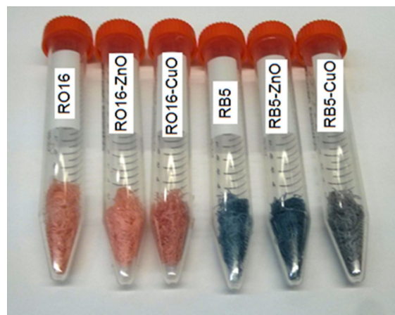
Figure 2: Images of textile fibers (shredded bandages) colored with RO16 and RB5 dyes and functionalized with ZnO and CuO NPs in a one-step sonochemical process.
