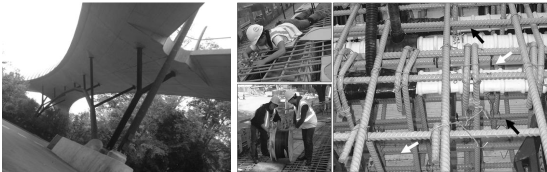
Fig. 18 Streicker bridge monitoring by DiTeSt system
