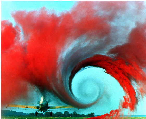
Turbulence in the tip vortex from an airplane wing. Studies of the critical point beyond which a system creates turbulence were important for chaos theory, analyzed for example by the Soviet physicist Lev Landau, who developed the Landau-Hopf theory of turbulence. David Ruelle and Floris Takens later predicted, against Landau, that fluid turbulence could develop through a strange attractor, a main concept of chaos theory.
