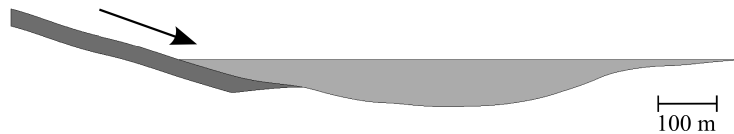
Figure 8. Landslide on Yesa reservoir. 2D model used for calibrating the PFEM parameters. The figure corresponds to the B-B' section in Figure 7.
