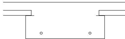
Figure 3.2 Finnish system of light steel composite construction
