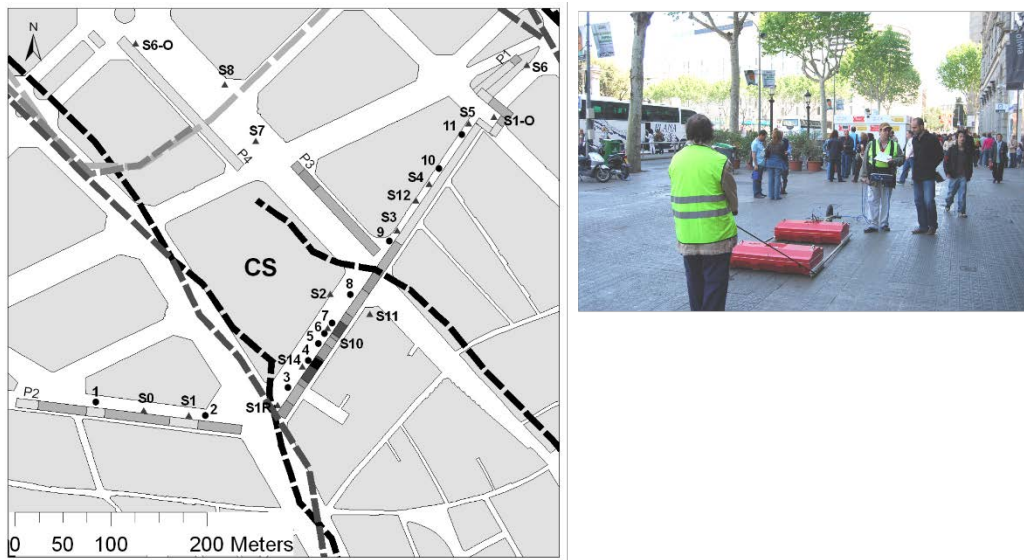
Figure 3. Site 1 in Catalonia Square (CS). Position of torrents according to different authors (in dashed lines from dark to clear: [Ventayol et al., 2000]; [Arandes, 1998]; [Vazquez, 1861]; [Cerde, 1855]). In continuous lines, position of the GPR profiles. Different colours indicate the noise amplitude due to scattering in GPR images (from dark to clear: very strong scattering, strong scattering, medium scattering, weak scattering and very weak scattering). Borehole: triangles. Old well: star. H/V amplification measurement points: numbers 1 to 11.
