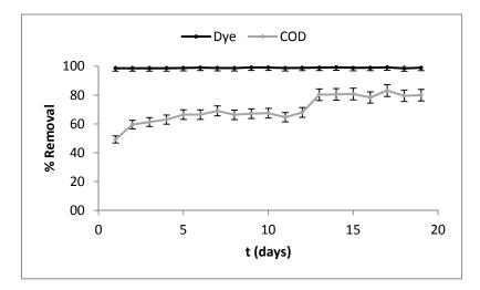
Figure 7- Dye and COD removal with ZW-1 membrane
