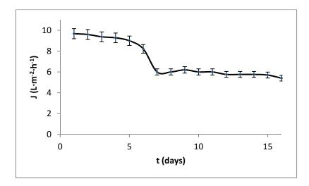
Figure 5- Flux values of U-1b membrane
