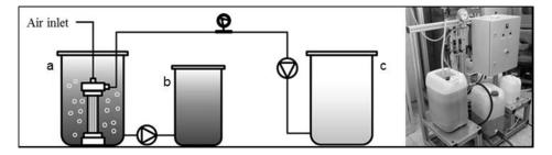
Figure 2- Pilot 2 with ZW-1 membrane. a) ZW-1 Membrane, b) Feed tank, c) Permeate tank
