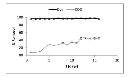
Figure 4- Dye and COD removal with U-1b membrane
