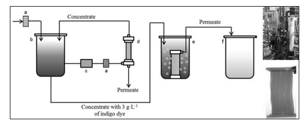
Figure 3- Semi-industrial system. a) Meshes, b) Feed tank, c) Control system, d) U-4 membrane, e) FP-T membrane, f) Permeate tank.
