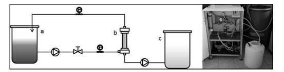
Figure 1- Pilot 1 with U-1b membrane. a) Feed tank, b) U-1b Membrane, c) Permeate tank
