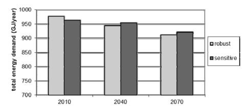
Figure 6. Total energy demand in Rome for the high emissions scenario prevision—one building  $40 \times 30 \times 9$  m<sup>3</sup>.
