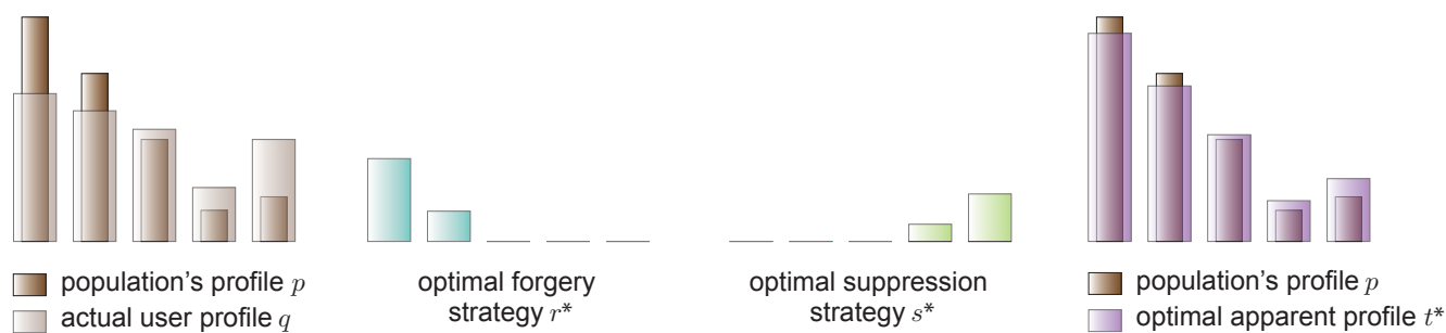
Figure 2. A user’s item distribution is perturbed according to two optimal forgery and suppression strategies, in order for the resulting profile to minimize the KL divergence with respect to the population’s distribution.
