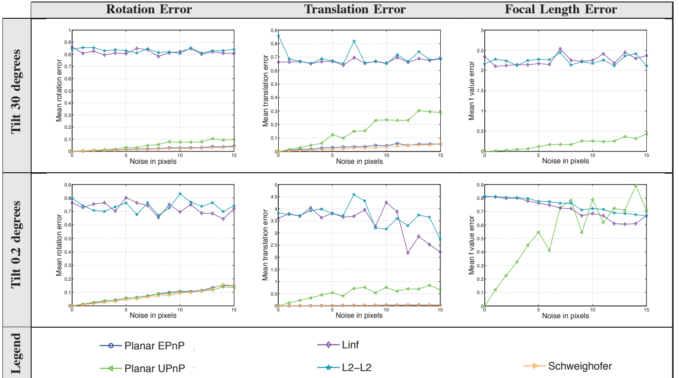
Fig. 7. Results on synthetic data for planar distributions of points. Mean rotation, translation and focal length errors for increasing levels of image noise, and two different tilt values.
