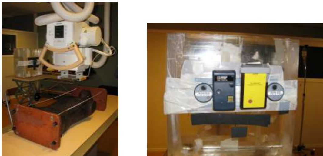
Figure 3.28: General set-up (left) and positioning of APDs and TLD reference on ISO slab phantom (right)
