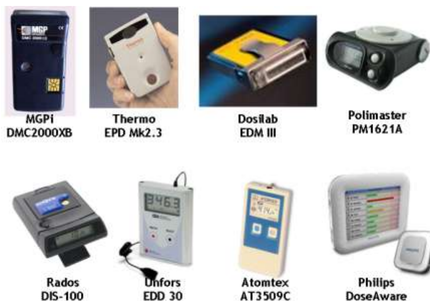
Figure 3.2: Active personal dosimeters tested in this study
