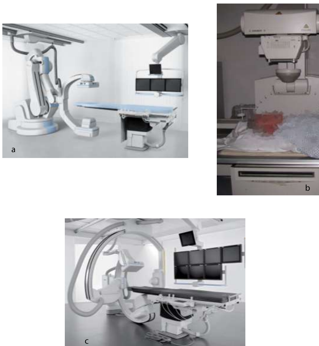
Figure 1.4: (a) Tube below configuration, (b) Tube above configurations and (c) bi-plane configurations
