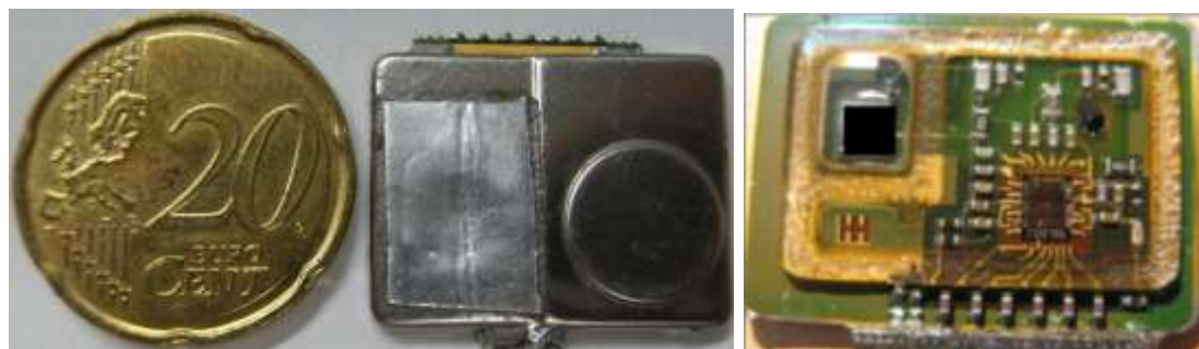
Figure 3.33: Prototype of detection module with and without shielding
