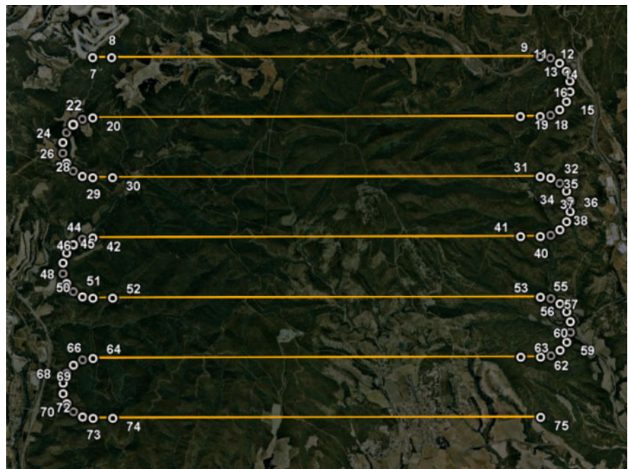
Fig. 9 Generated waypoints for a scanning pattern
