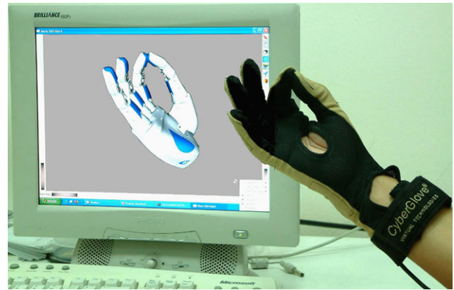
Fig. 6 Human hand with the sensorized glove connected to the mechanical hand simulator
