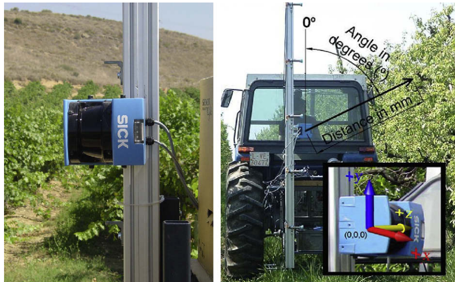
Fig. 1 – LIDAR system for field test in vineyard (left) and pear orchards (right), also showing polar (distance, r , and angle, \theta ) and Cartesian ( x,y,z ) coordinates reference systems.
