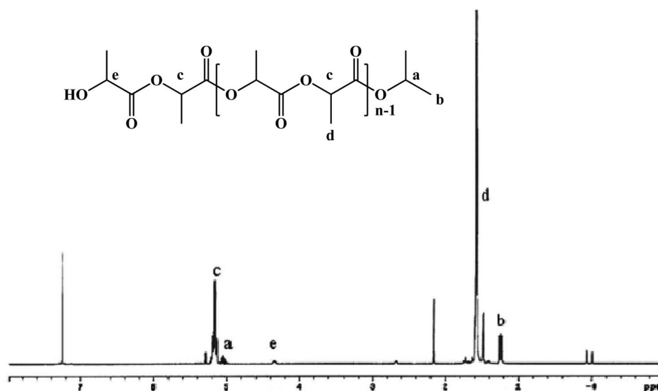
Fig. 4 ^1\text{H} NMR spectrum of PLLA-50 (50 indicates [\text{LA}]_0/[\mathbf{1}]_0 = 50 ).
