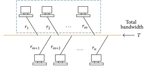
FIGURE 1: The system bandwidth allocation  $\mathbf{r} = (r_1, r_2, \dots, r_n)$  subject to user-wise constraints:  $r_i \leq r_i \leq \bar{r}^i$  for  $i \in \{1, 2, \dots, n\}$ , and a user-grouping constraint  $R_g \leq \sum_{i=1}^m r_i \leq \bar{R}_g$ . The total allocation  $R = \sum_{i=1}^n r_i$  is less than  $T$ , the total bandwidth.
