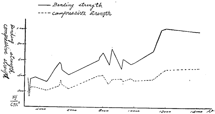
圖 2: 單位面積內細胞壁所占面積與抗彎強及抗壓強之關係。 Fig. 2: The sectional area of cell wall in unit area in relation to bending strength and compressive strength.
