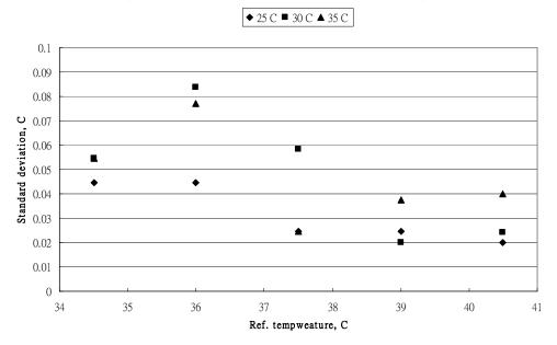
At the standard temperature of 36 °C, the standard deviations for three ambient temperatures were higher than that of other standard temperatures. To evaluate the factors affecting the standard
