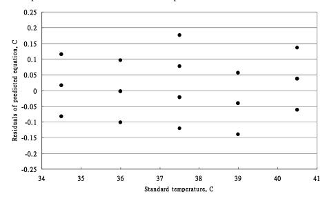
Figure 6. The predicted errors of calibration equation of BRAUN IRT-3020 thermometer.
