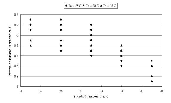
The relationship between standard temperature values and reading values of MC-510 thermometer was established by regression analysis. The best equation is:
