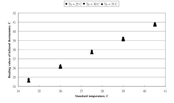
**Figure 5.** The error distribution of BRAUN IRT-3020 thermometer at three ambient temperatures.
