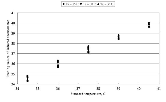
**Figure 2.** The error distribution of OMRON MC-510 thermometer at three ambient temperatures.
