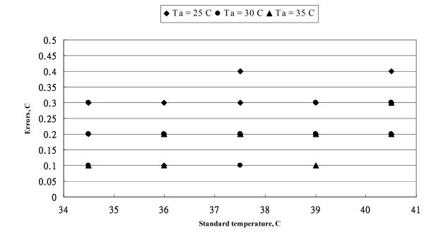
The relationship between standard values and reading values of IRT-3020 thermometer was established by regression analysis. The adequate equation is:
