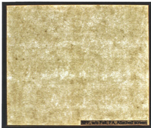
Figure 145. A sheet made with unfermented flax, without felt, with mucilage, and with a fixed laid screen.
