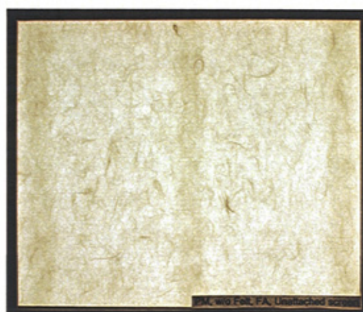
Figure 142. A sheet made with paper mulberry, without felt, with formation aid and with a flexible screen.
