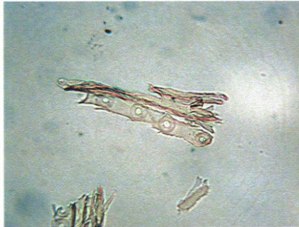
Figure 116. Clear bordered pits in broken wood fibre (x250) from British Library Korean collection, Or6998(10-5) in 1778.
