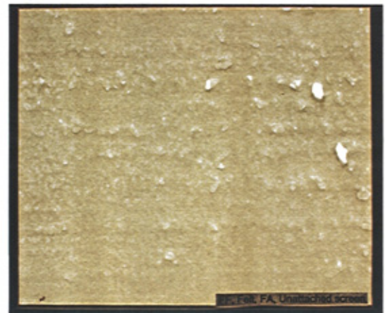
Figure 150. A sheet made with fermented flax, with felt, with formation aid, and with a flexible screen.
