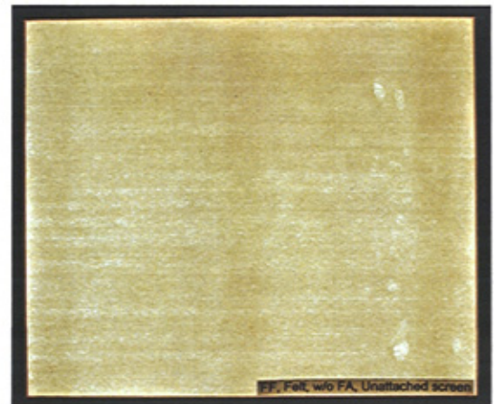
Figure 148. A sheet made with fermented flax, felt, without formation aid, and with a flexible screen.
