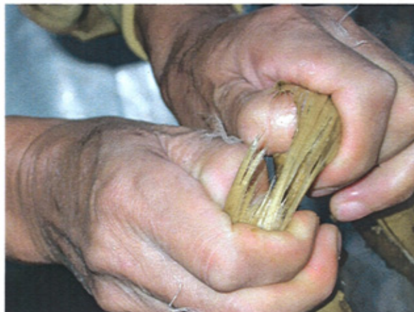
Figure 23. A papermaker checking the cooked baekpi (the picture was taken at Jangjibang, in Korea)
