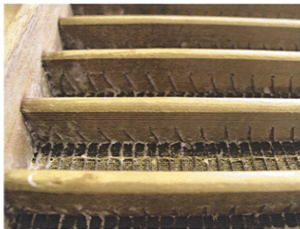
Figure 9. Close-up of the supporting ribs in Figure 6. The picture shows the detailed construction of the wove mould.
