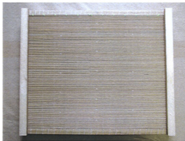
Figure 91. A fixed laid screen – a bamboo screen was fastened to its supporting frame with thread. Two deckle sticks were also placed on the vertical edges of the screen.
