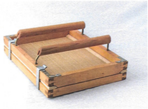
Figure 16. A flexible laid screen is in place and the assembly is locked with two metal clips.
