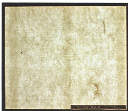
Figure 141. A sheet made with paper mulberry, without felt, with formation aid and with a fixed screen.
