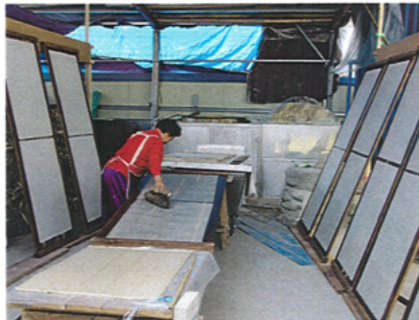
Figure 33. Placing wet sheets on a wooden drying board (The picture was taken at Sinhyeonse Hanji, in Korea).
