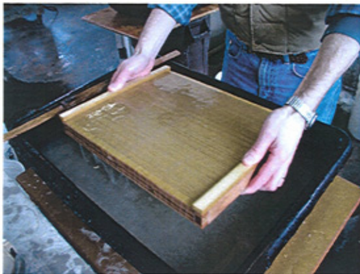
Figure 95. Sheet forming with a fixed screen mould, paper mulberry and formation aid.
