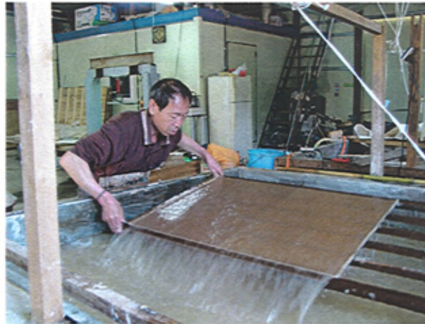
Figure 30. Casting off the excess stock (during sheet forming process, the picture was taken at 'Sinhyeonse Hanji' in Korea)
