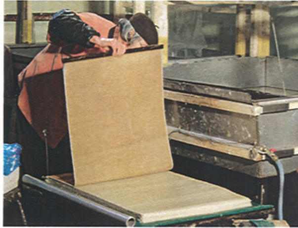
Figure 31. A papermaker couching a newly formed sheet onto the pile of the previously couched sheets. (The picture was taken at Jangjibang in Korea)
