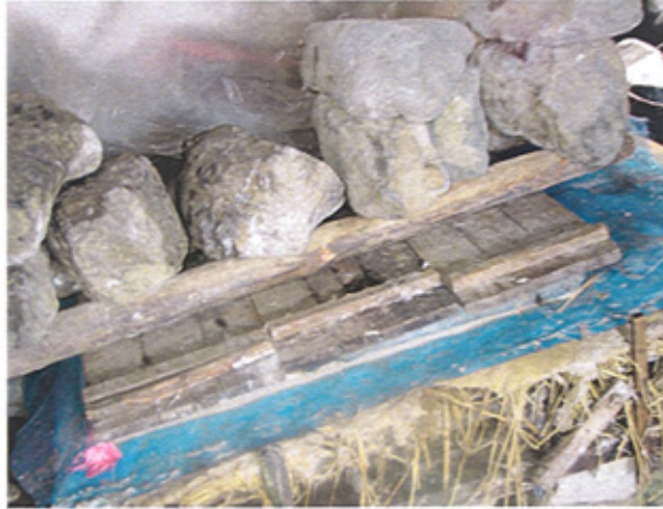
Figure 32. A pile of sheets covered with a wooden board and pressed with heavy stones (The picture was taken at a traditional paper mill in Jeonju, Korea).
