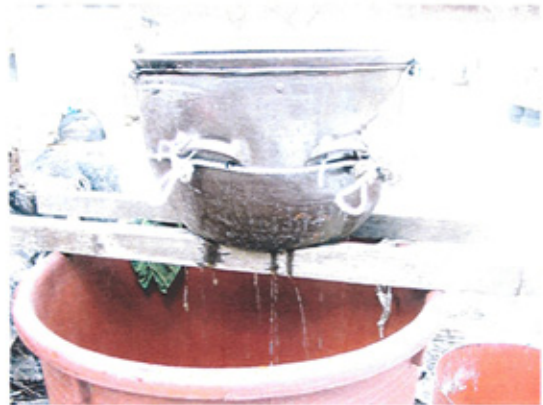
Figure 22. Collecting the alkali solution. (The picture was taken at Jangjibang in Korea)
