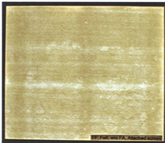
Figure 147. A sheet made with fermented flax, felt, without formation aid, and with a fixed screen.
