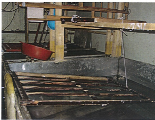
Figure 14. A Korean style mould (without screen) being placed in the vat (photo taken at Jangjibang, a traditional papermaking mill in Gapyeong, Korea).
