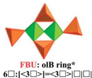
Fig. 17 The FBU 6\Box:\Box<3\Box>=\Box<3\Box>\Box\Box\Box contains only borate tetrahedra with a connectedness Q^{n/CN} = B^{4/4} and can not further be condensed due to the terminal character of the phosphate groups.
