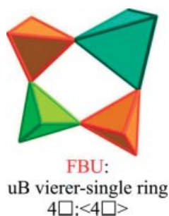
Fig. 29 An unbranched vierer-single ring [\text{MBP}_2\Phi_{13}] (MPBP) represents the common fundamental building unit of metalborophosphate partial structures.
