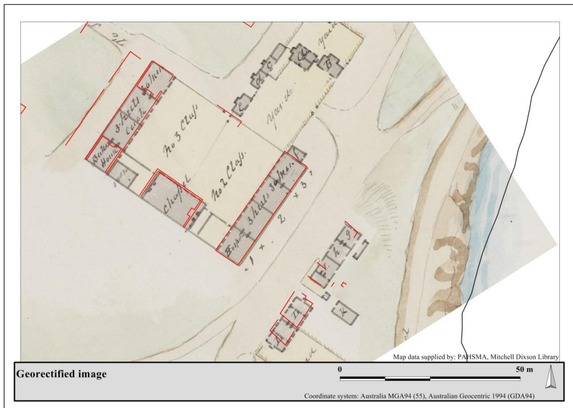
Figure 4-3: Excerpt from the 1842 probation plan showing the image georectified against the 2008 survey data (red)
