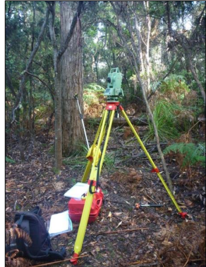
Total Station used during the survey
