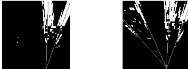
Figure 1.6: Correspondence between triangles and directions pointed out by peaks detected in the polar histogram.
