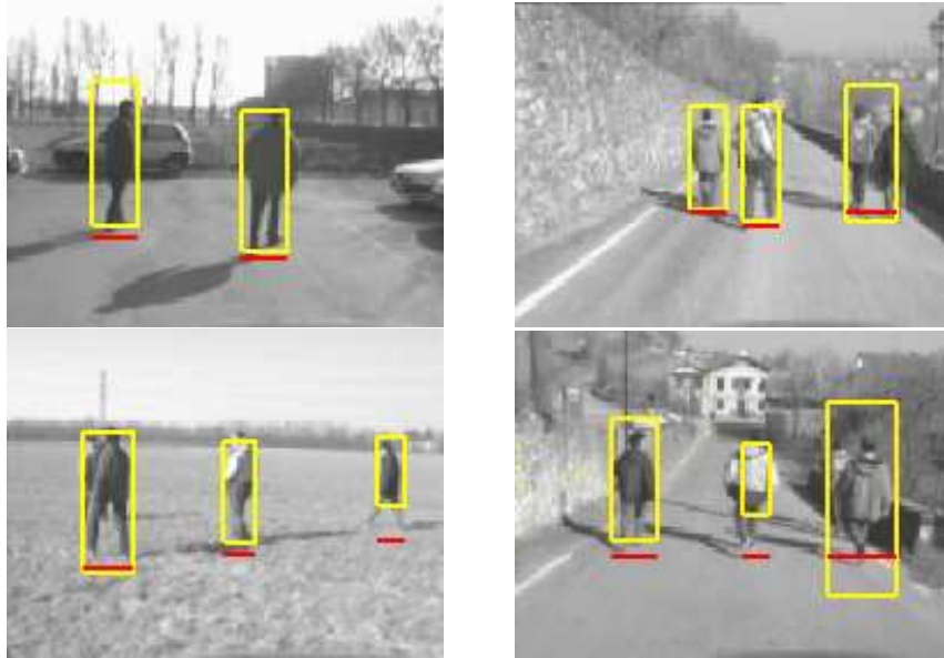
Figure 4.4: Stereo refinement: the yellow bounding box is generated during the symmetry detection, the red line represents the stereo refinement of the box's bottoms.
