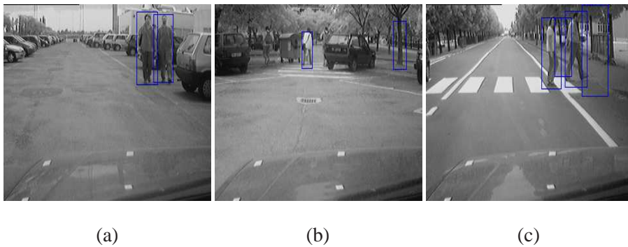
Figure 1.16: Result of low-level processing in different situations: (a) a correct detection of two pedestrians (b) a complex scenario in which only the central pedestrian is detected; the left one is confused with the background, the right one is only partially visible, while the high symmetry of a tree has been detected as well; (c) two crossing pedestrians have been localized, but other symmetrical areas are highlighted as well.
