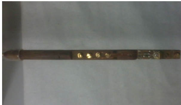
Figure II.22. Ending part of the capacitance probe for dielectric characterization within the SQuID magnetometer.
