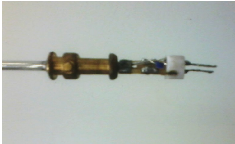
Figure II.23. The inner part of the probe devoted to pyroelectric measurements within the SQuID. The outer cylindrical screen, made of non-magnetic brass material, has not been included in the picture.
