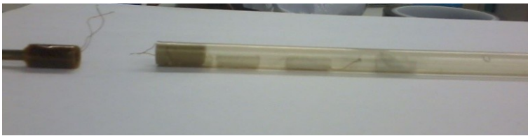
Figure II.24. The insulated and screened magnetolectric probe which houses the metalized sample. This asset allow to apply DC electrical poling up to 105 V.
