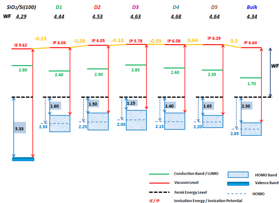
Figure 6.48: Energy level scheme of Si(100) substrate, H 2 TPP(F) thick film and D1, D2, D3, D4, D5 samples. Organic film IP, WF, and the extrapolated LUMO position are displayed. The HOMO band and centroid position are also illustrated. All values are in eV.
