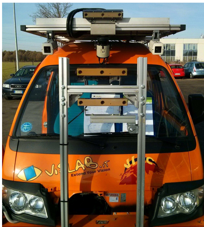
Figure 4.1: Cameras setting on a VisLab vehicle (Porter) used during the VIAC.
