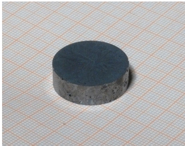
Figure 3.1: Typical 1" diameter CIGS target for PED synthesized at IMEM.
