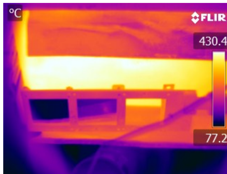
Figure 3.5: Thermo-image of two samples before the CIGS deposition
