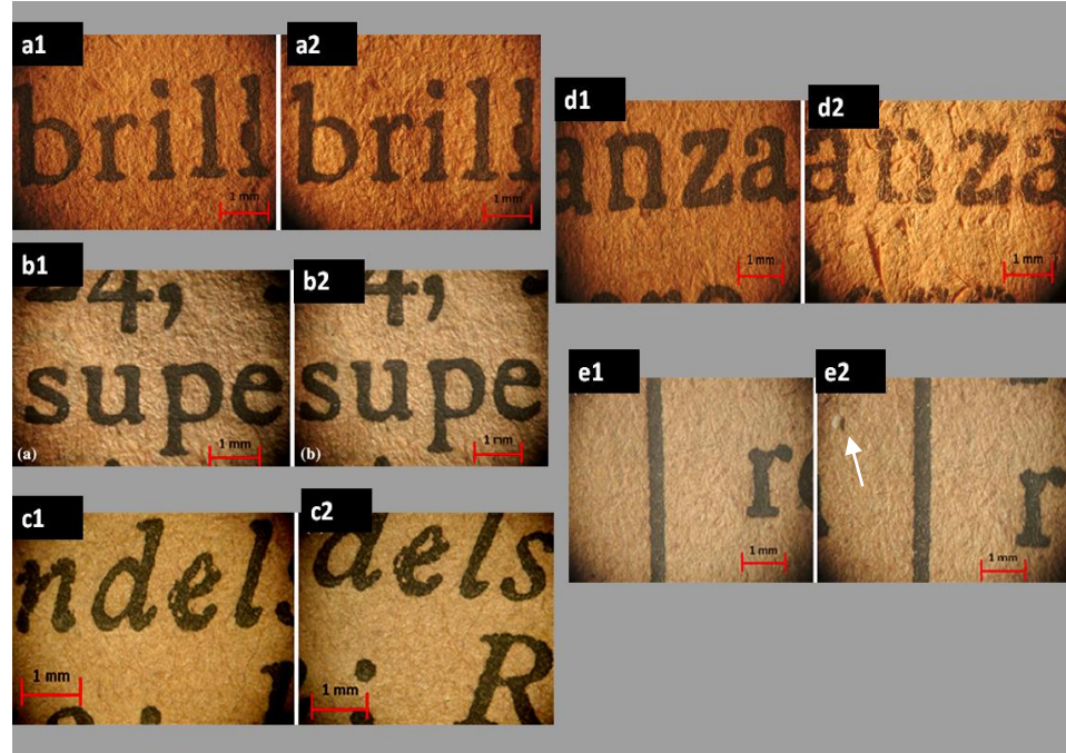
Figure 4.3: Stereo-microscopy observation of paper samples: gellan gum 2% treatment (a1= before; a2=after the treatment); agar gel 2% treatment (b1=before; b2= after the treatment); washing by immersion in distilled water treatment (c1= before; c2= after the cleaning treatment); Klucel G ® 2% application (d1= before; d2= after the treatment); cleaning treatment with Wishab ® sponge (e1=before; e2= after the treatment) (x10 magnification; x4 zoom camera).
