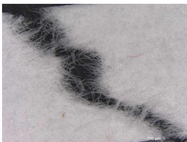
Figure 3.36: Stereo-microscope observation of tensile failure of sample treated with agar gel 1% (A1-0h) (magnification: 8x). Sample presents a granular morphology.
