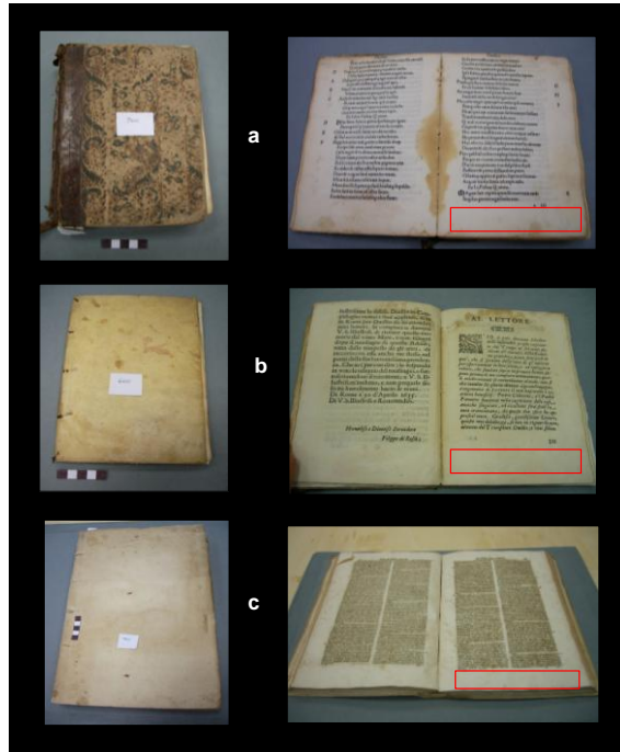
Figure 6.1: Paper samples from 16 th century (a), 17 th century (b), 18 th century (c) books and sampling areas (red frame).
