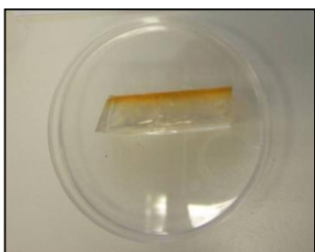
Figure 1.22: Observation of gellan gum gel 2% (w/v) in section after application on a 17 th century paper for the cleaning treatment. A yellowing of the gel is observed after the application on paper caused by the migration of degradation products, organic acids from paper to the gel structure.
