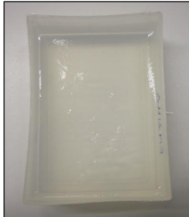
Figure 1.24: Agar rigid gel 2% after gelation.
