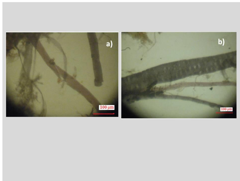
Figure 4.1: Fibres of cotton a) and wood b) of paper sample after the treatment with Herzberg reagent (x100 magnification; x4 zoom camera).
