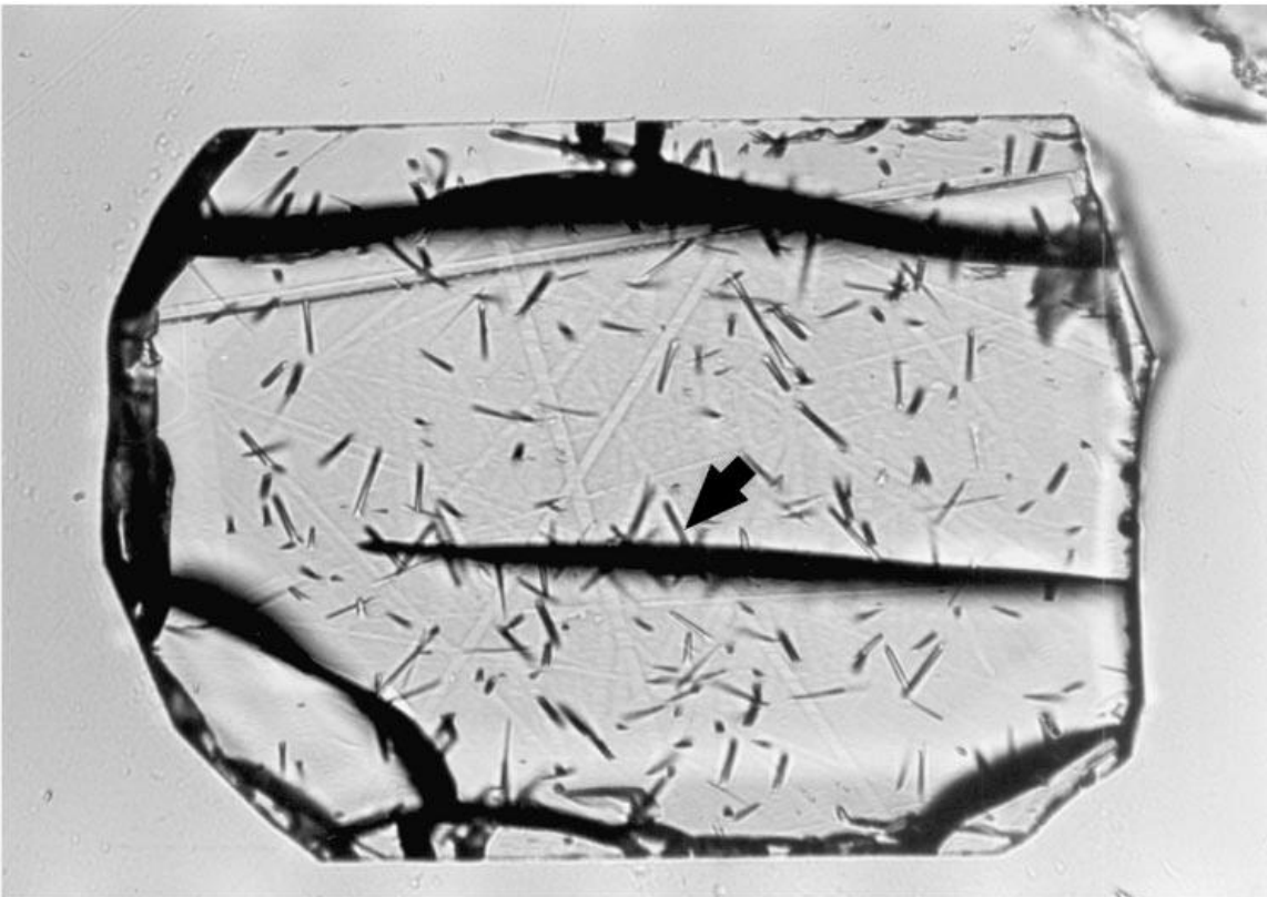
Fig. 4.6 – Photomicrograph of a polished and etched prismatic section through an apatite crystal. The arrow indicates the intersection between an etched surface and a horizontal confined track (after Gallagher et al., 1998).
