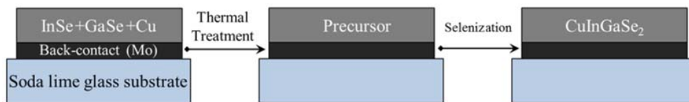
Figure 52. Schematic image of the second method developed for CIGS deposition, using InSe, GaSe and Cu starting materials.
