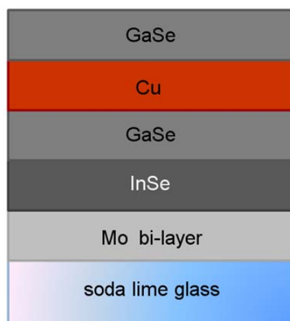
Figure 59. Scheme of the precursor structure final version.
