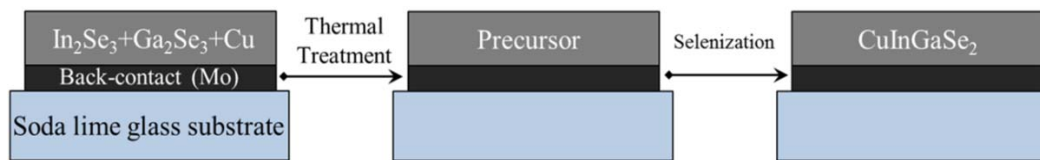
Figure 48. Schematic image of the second method developed for CIGS deposition, using \text{In}_2\text{Se}_3 , \text{Ga}_2\text{Se}_3 and Cu starting materials.
